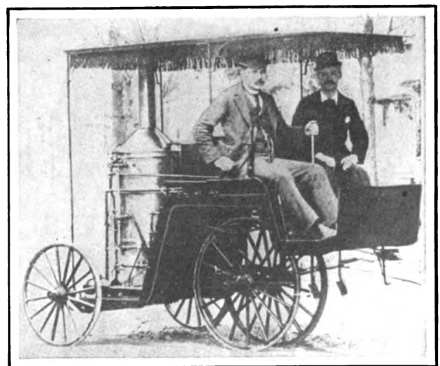
R. E. Olds in his second steam car built about 1890. Note the double front wheel steer. The same rear wheels and axle were used in his first design
